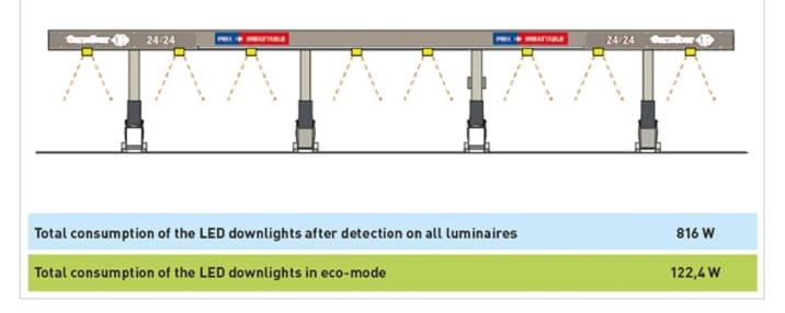
When customers are entering the fuel station and motion is detected, all LS Downlights will go to full power to ensure a safe environment and optimal visibility:
