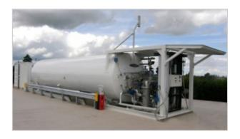
The resultant product, LNG DYNAFLOW 3000® Dispenser, fuels heavy duty trucks and buses with LNG, reliably, accurately, safely and quickly.
