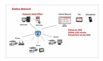
Optavias Basis is the proven PC solution that enables you to poll Hectronic gauges at filling stations and visualise tank data. Based on this system, Optavias Head Office centrally retrieves tank data from all connected filling stations via modem or the Internet. Provided that all filling stations are equipped with Mineo Controllers, Maxam Controllers or Optavias Basis. The polling frequency is easy to configure in accordance with your individual requirements.
