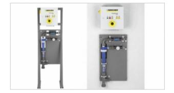
Cost savings thanks to low maintenance requirements – this is what the new WRP Car Wash compact water recycling system for car washing bays has to offer. The water is reprocessed using a cyclone which separates the particles of dirt from the washing water. With a flow performance of up to 3,000 litres per hour, the system is suitable for all car washing bays in car dealerships, workshops, service stations and service centres which use reprocessed water.
