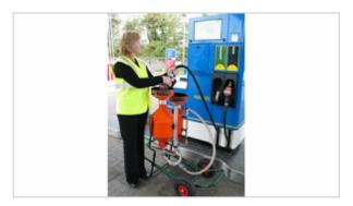
The resulting improved ergonomics allow the safe use of larger capacity measures and raise fundamental questions as to the appropriate size of samples for inspection and verification of dispensers and the validity of minimum delivery and slow flow rate tests. Are the use of 2, 5 and 10 litre measures, minimum delivery and slow rate tests relevant to the typical use of fuel dispensers and to consumer protection?
