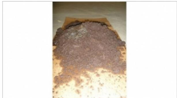
Figure 2: Bacterial sludge removed from a tank system as a result of water ingress
