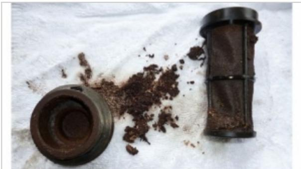
Figure 1: Microbial contamination led to corrosion and blockage of filters at this site 18 months after it opened
