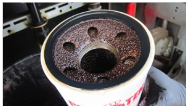
Corrosion on the inside of a filter removed from diesel dispenser
