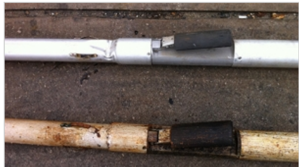
A corroded flapper valve from a diesel tank, next to another flapper valve from the gasoline tank at the same site
