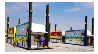
Totem signs of 12 metres height, painted to match existing columns and structures in the surroundings, were made of steel I-section. Similarly, a variation of entry and exit signs, traffic signs, facility units, c-store signs and graphics were custom-produced to coordinate with the prevailing theme.
