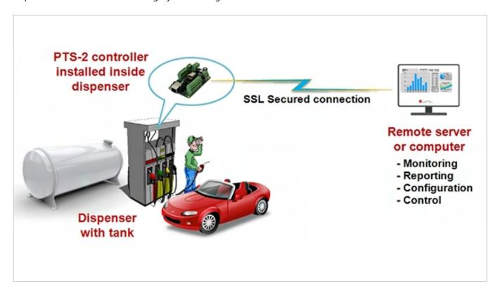
This small device supports more than 110 brands of fuel dispensers and 40 brands of tank monitoring systems and probes. It can provide simultaneous control over up to 50 fuel dispensers and monitor up to 50 tanks. It can also communicate with any POS and control systems (OPT, cash registers) and remote servers at the same time, which is often needed at big petrol stations.
