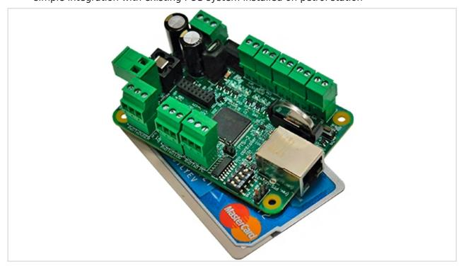
All this is possible with PTS-2 forecourt controller. It is a miniature controller, with a size of a credit card, but packed with great functionality. Due to its small dimensions, the PTS-2 forecourt controller can be easily mounted inside any fuel dispenser housing in order to provide control over all fuel dispensers and tank monitoring systems of gas stations.
